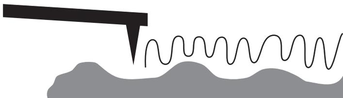
**Figure h.** In vibrating methods, changes in probes vibrations are monitored to establish the force of the probe onto the surface.
