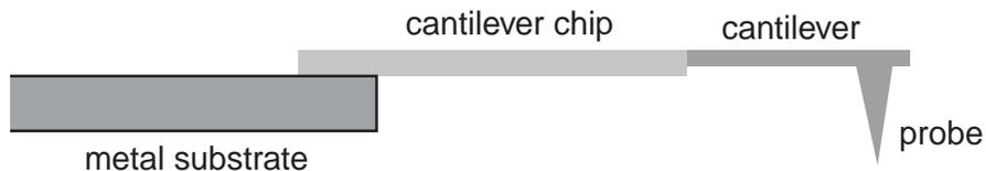
**Figure 1.6.** PNI AFM probe (side view—not to scale).
