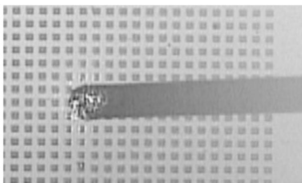
**Figure 2.26.** Centering the laser spot on the cantilever.
