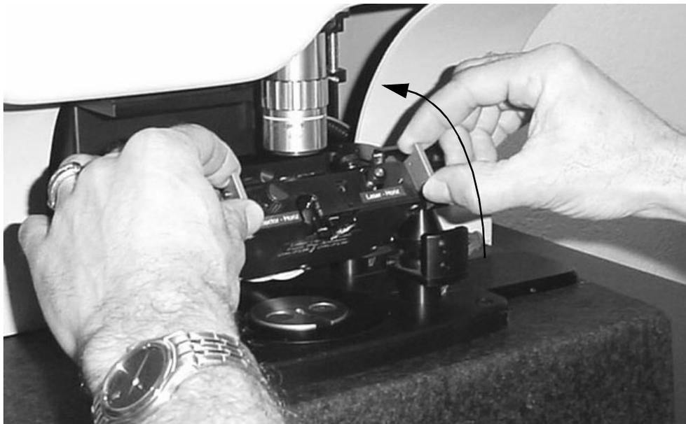
**Figure 2.17.** Rotate the scanner head.
