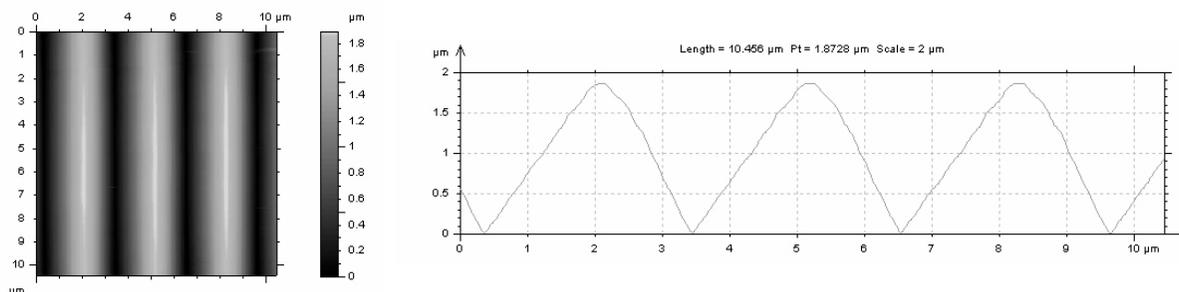
**Figure A.20.** AFM image of a sample with a repeating triangle pattern and the extracted line profile.
