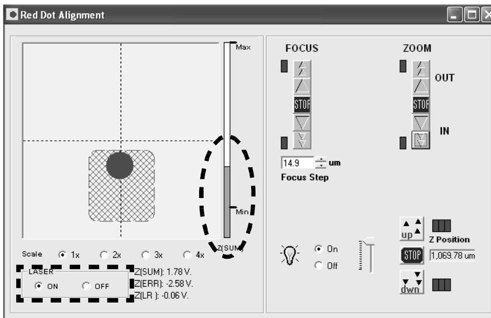
Figure 2.27. Aligning the detector.
