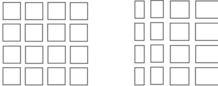
**Figure A.9.** A test pattern of squares (left) will appear severely distorted (right) if the piezoelectric scanner in the AFM is not linear.
