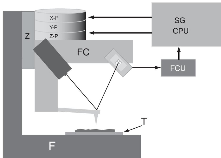
**Figure e.** Main components and subsystems of an AFM system.
