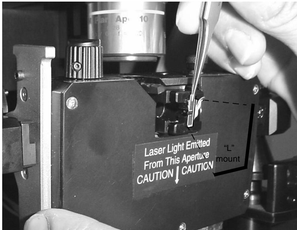
**Figure 3.20.** Mounting the probe.
