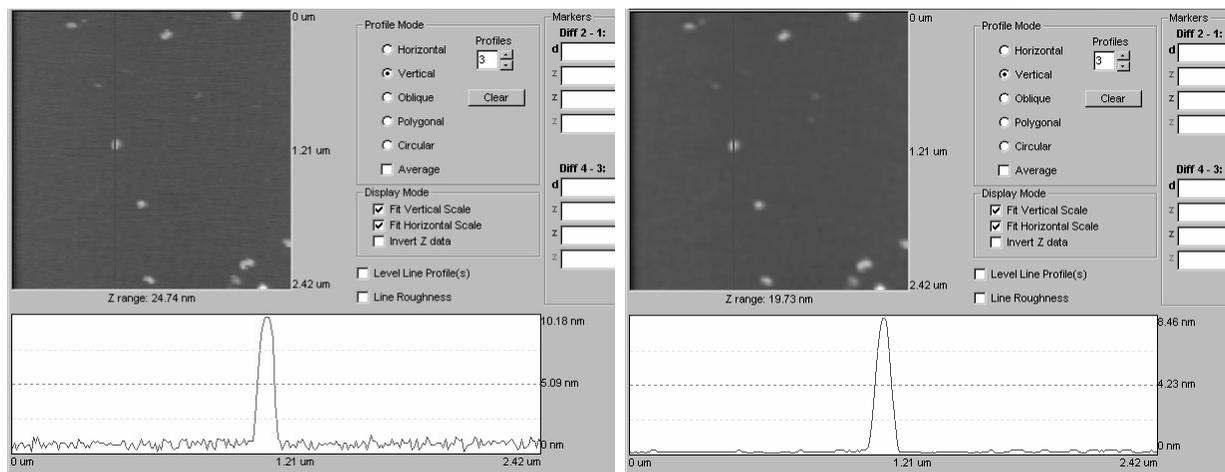
**Figure A.23.** AFM image of nanospheres before and after matrix smoothing.
