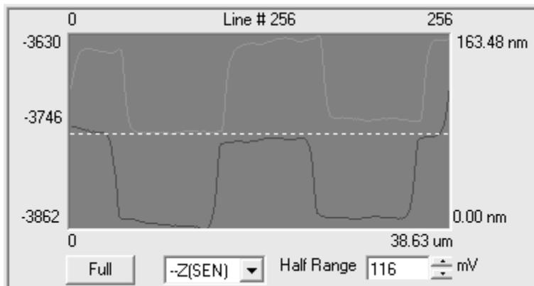
**Figure 2.35.** Viewing a single line scan.
