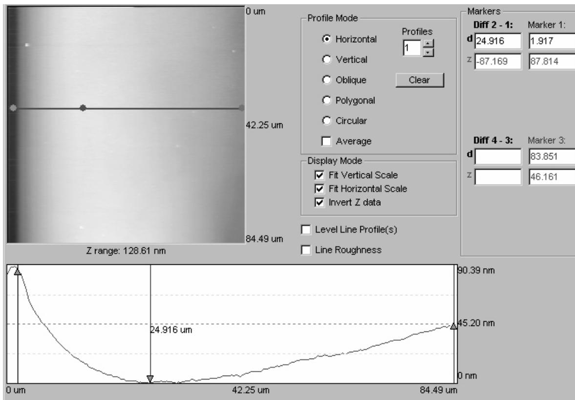
**Figure A.13.** Bow in AFM image and line profile of a flat piece of silicon. Scan size: 85 X 85 μm.
