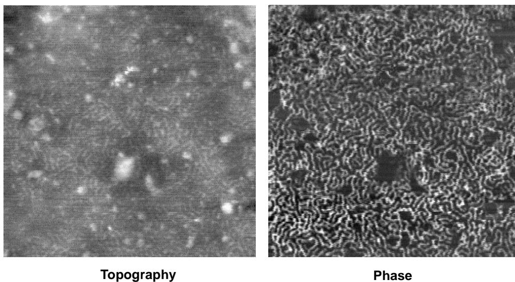
**Figure 4.5.** 1.5x1.5  $\mu\text{m}$  image of SBS film.
