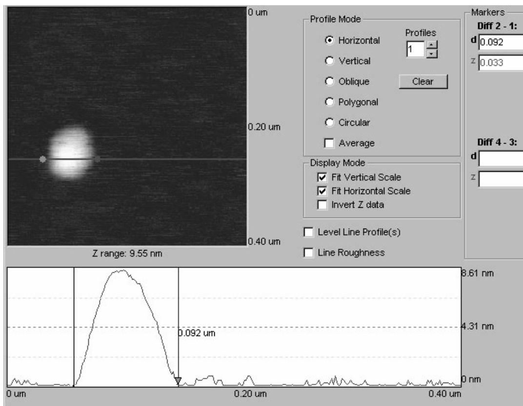
**Figure A.2.** AFM image and line profile of an 8 nm diameter sphere. Scan size: 400 X 400 nm.
