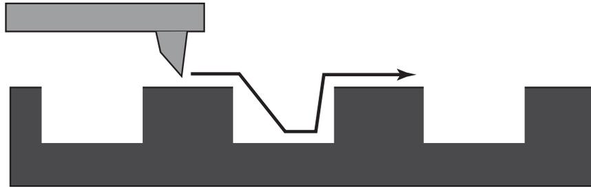
**Figure A.5.** Chipped AFM probe scanning over a sample surface.
