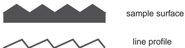
**Figure A.19.** Asymmetry caused by mechanical coupling between Z and X or Y piezoelectric ceramics.
