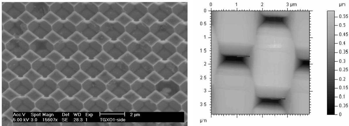
**Figure A.4.** SEM (left) and AFM (right) images of a test pattern of squares (NT-MDT TXO1).
