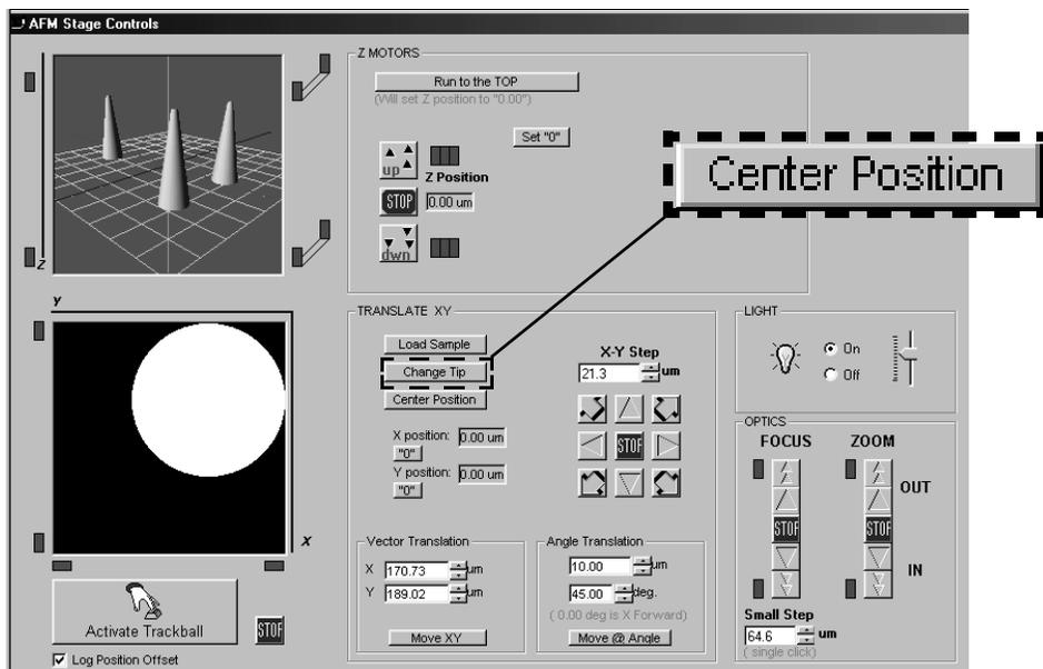
**Figure 2.12.** Return sample puck to initial X-Y position.
