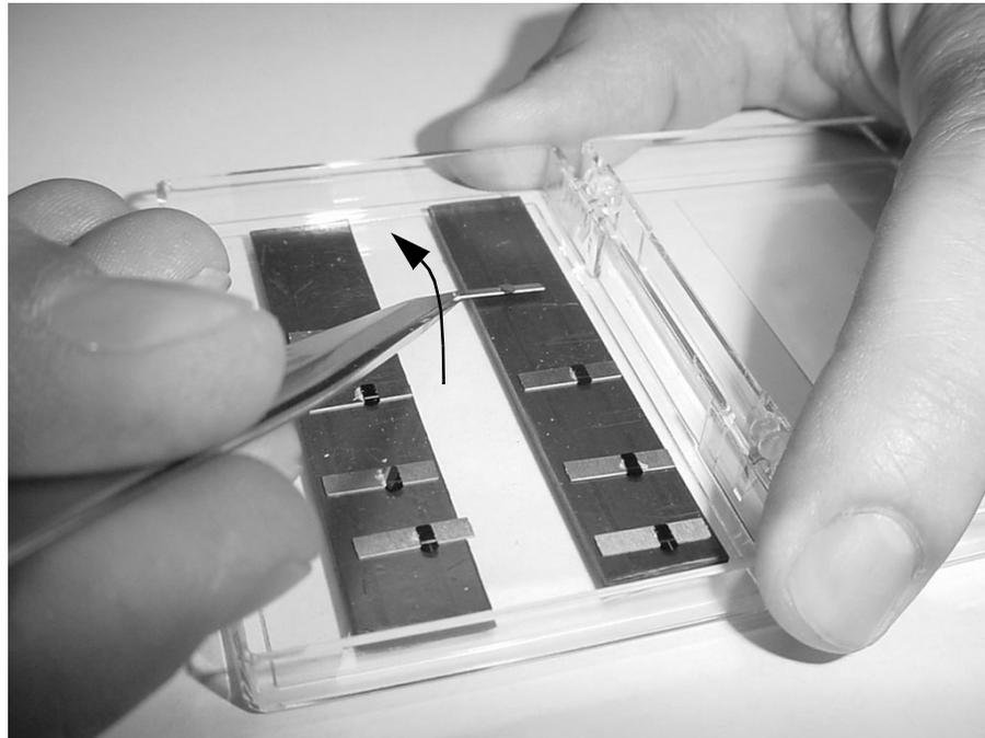
**Figure 2.21.** Lift the probe, cantilever side first.
