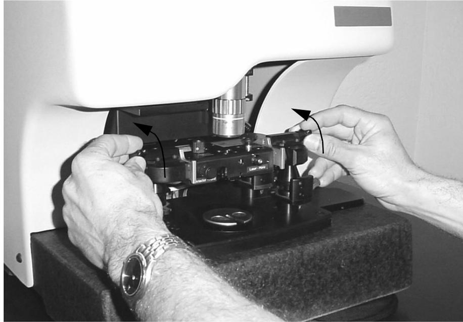
**Figure 3.13.** Turn the knobs to disengage the scanner head.
