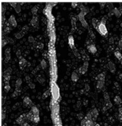
**Figure A.24.** AFM image of a nanotube showing “nodules” due to filtering. Scan size: 850 X 850 nm.
