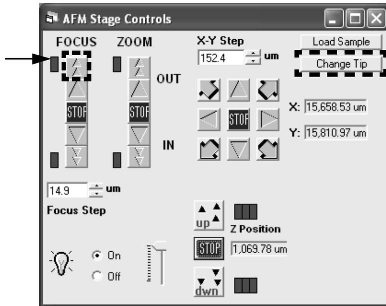
**Figure 2.13.** Raise the probe tip away from the sample.
