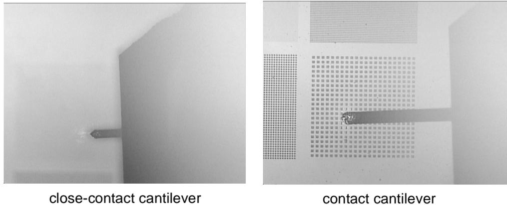
**Figure 3.23.** Contact vs. close-contact probes.
