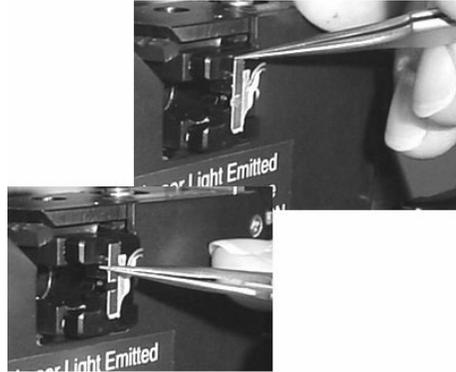
**Figure 2.23.** Push the probe substrate flush against the “L” mount.
