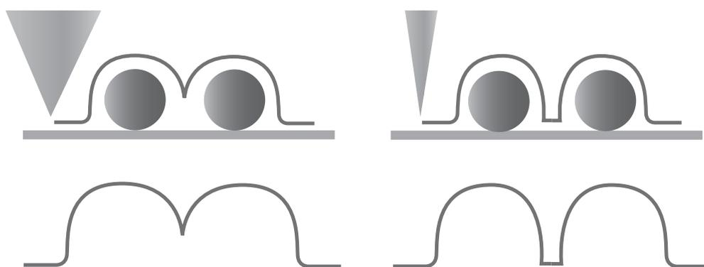
**Figure f.** Using a dull probe vs. a sharp probe to measure spherical features.
