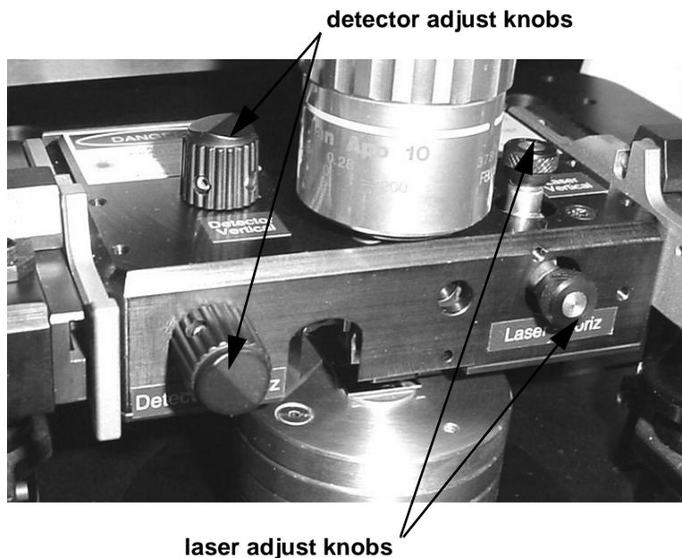
**Figure 1.4.** Adjustment knobs for laser and detector.
