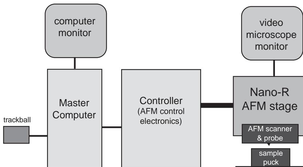
**Figure 1.1.** Block diagram of Nano-R instrument system.
