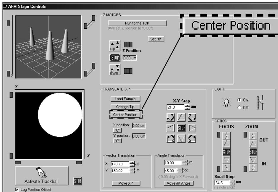
**Figure 3.10.** Return sample puck to initial X-Y position.
