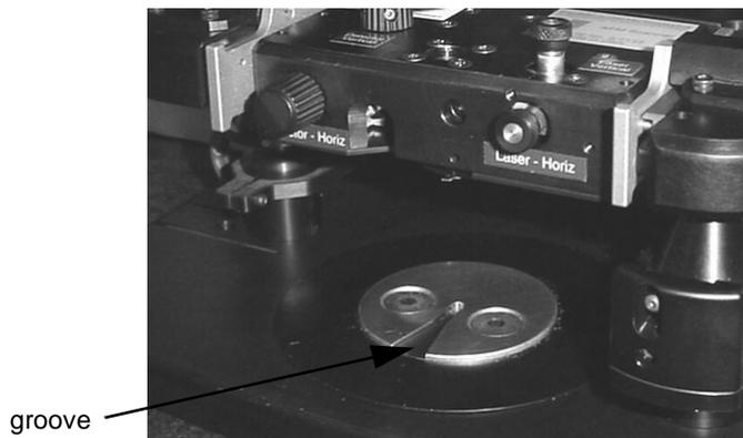
**Figure 2.11.** Fit the sample puck into the groove on the X-Y stage.
