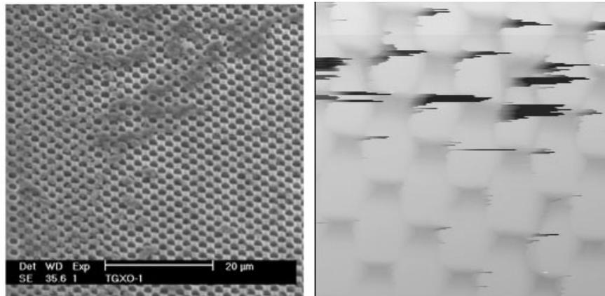
**Figure A.27.** SEM image (left) and AFM image (right) of a contaminated test pattern.
