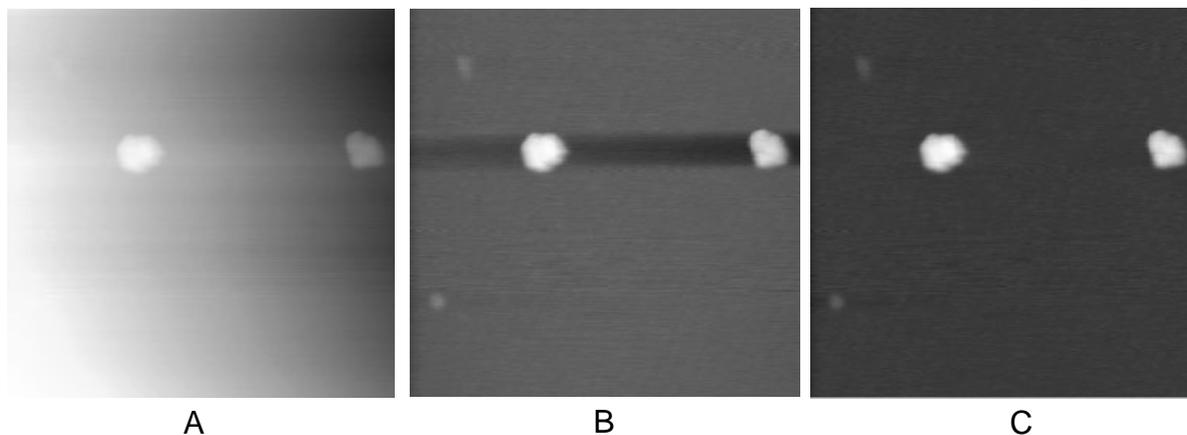
Figure A.21. Leveling of a 1.6 X 1.6  $\mu\text{m}$  AFM image of nanospheres.
