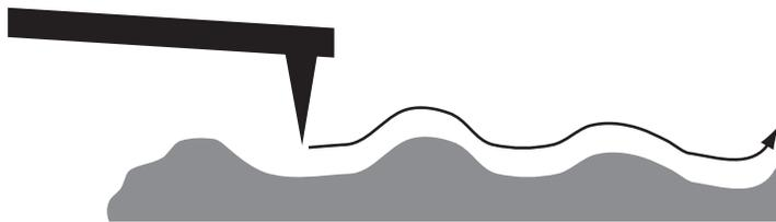
**Figure g.** Contact mode AFM: the probe directly follows the topography of the surface as it is scanned while a constant force is maintained.
