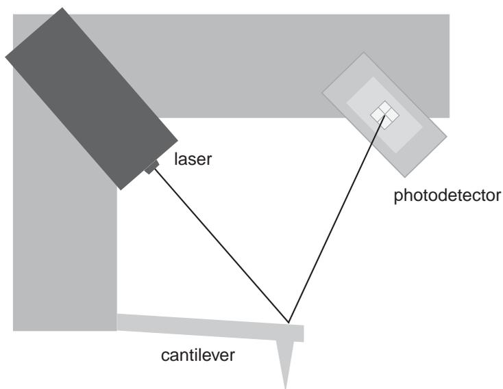
**Figure d.** The light lever method for sensing the motion of the cantilever.
