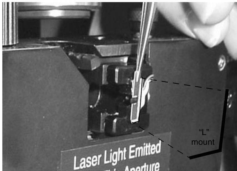
**Figure 2.22.** Mounting the probe.
