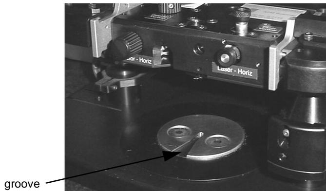
**Figure 3.9.** Fit the sample puck into the groove on the X-Y stage.
