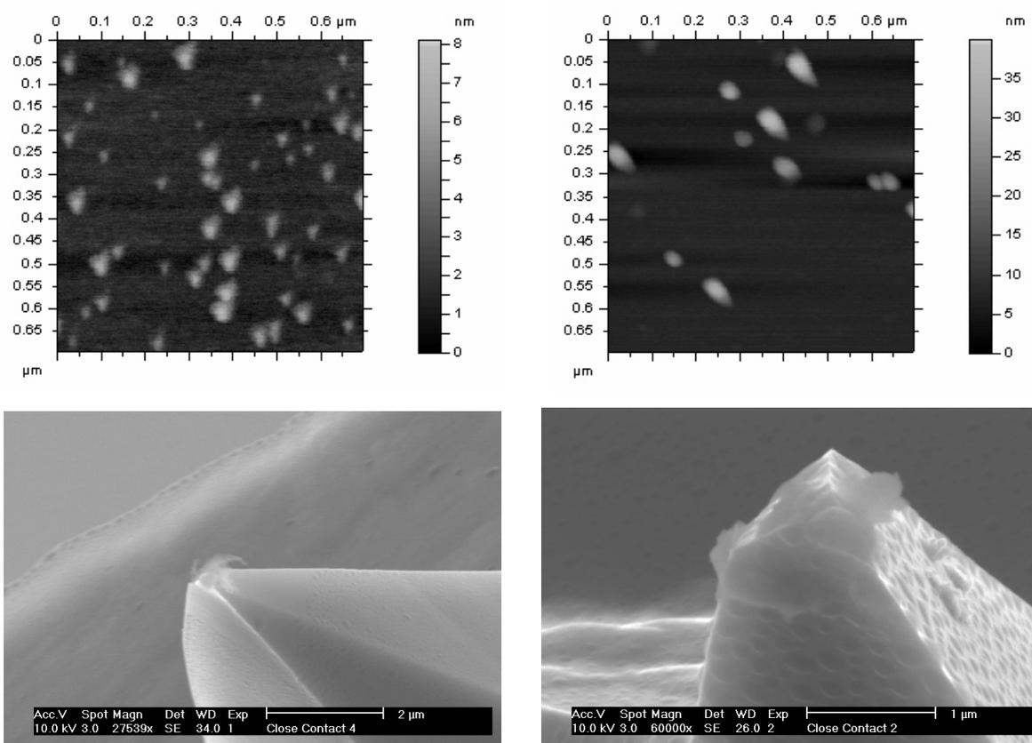
**Figure A.7.** AFM images of nanospheres (top) and SEM images of the probes used (bottom). Diameter of nanospheres: 5 nm (left) and 28 nm (right). Scan size: 700 nm X 700 nm.
