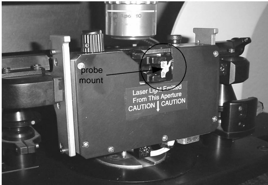
Figure 3.16. Probe exchange position.
