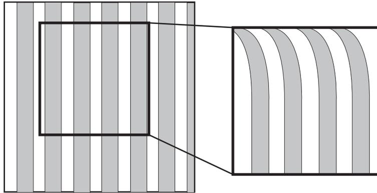
**Figure A.16.** Distortion due to drift in the initial part of a scan of a zoomed-in area.
