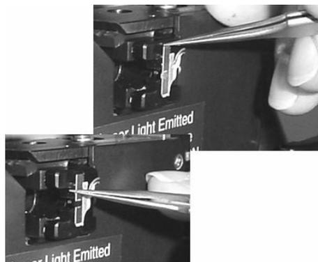
**Figure 3.21.** Push the probe substrate flush against the “L” mount.
