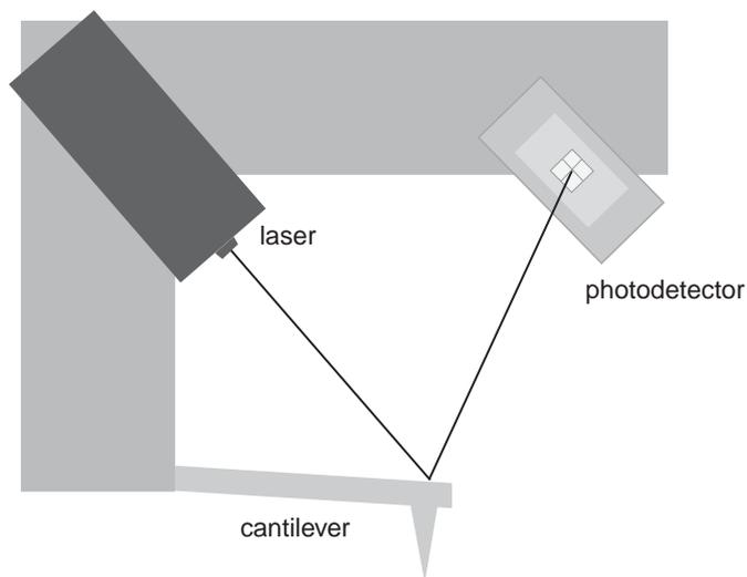
**Figure 1.3.** Light lever sensing system.
