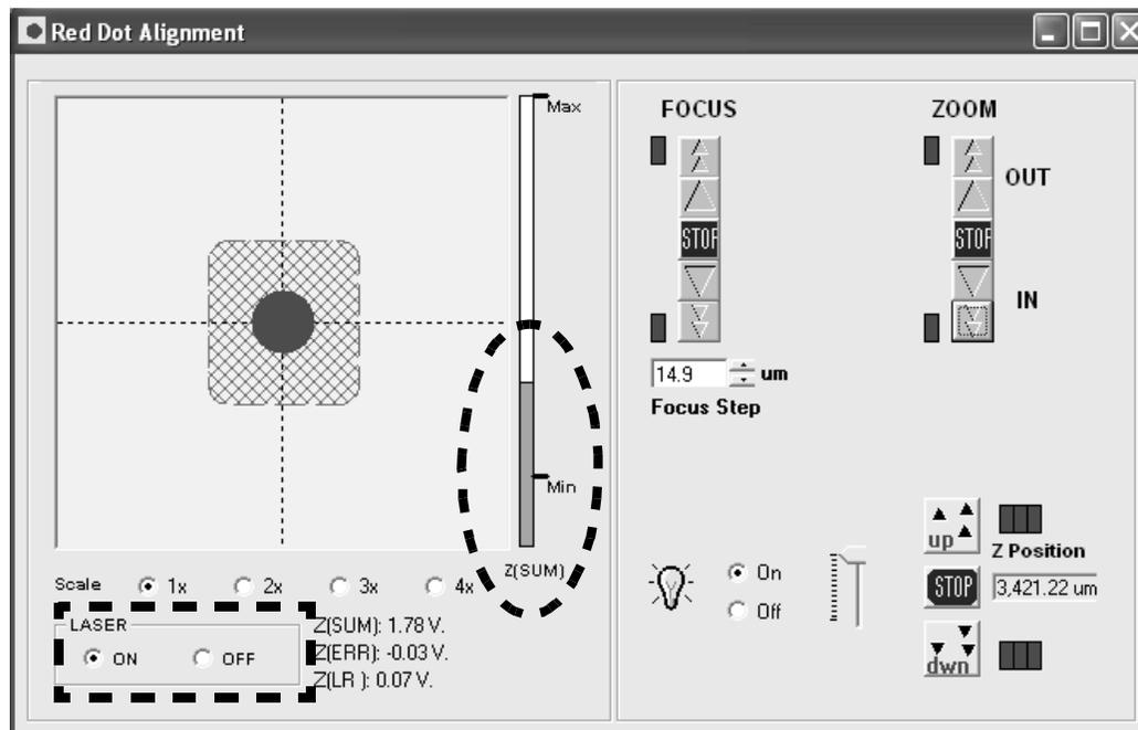
Figure 3.25. Aligning the detector.
