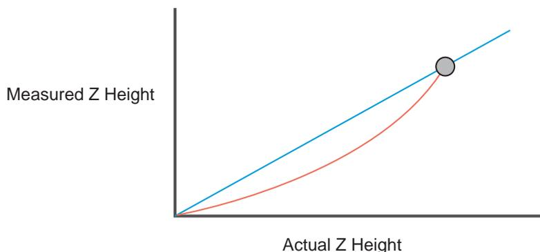
**Figure A.11.** Z calibration at only one point.
