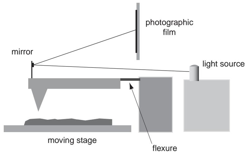
**Figure a.** Example of a surface profiler made in 1929.
