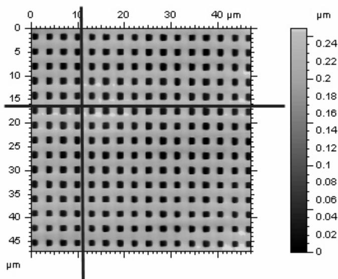
**Figure A.18.** AFM image of a test pattern with lines drawn to measure any error in orthogonality.
