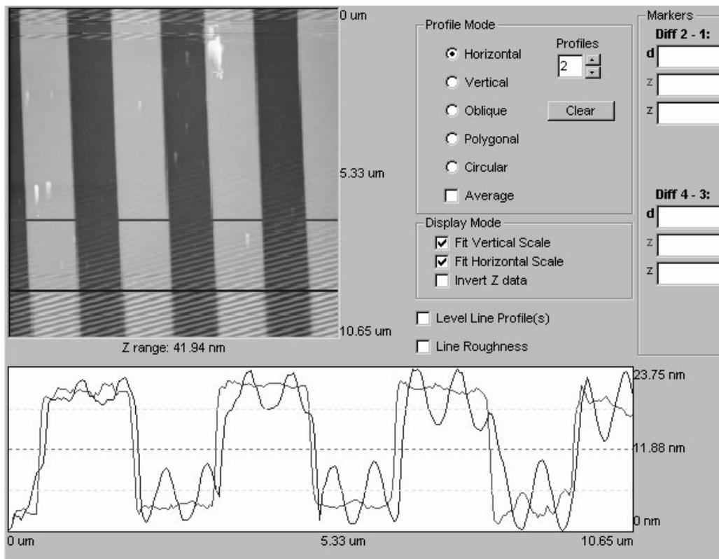
**Figure A.26.** Test pattern image with electronic noise at the top and bottom of the scan.
