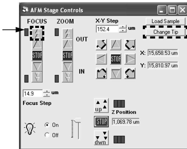
**Figure 3.11.** Raise the probe tip away from the sample.
