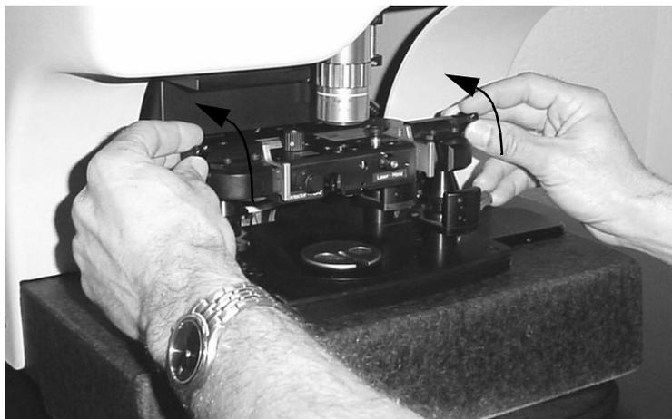
Figure 2.15. Turn the knobs to disengage the scanner head.
