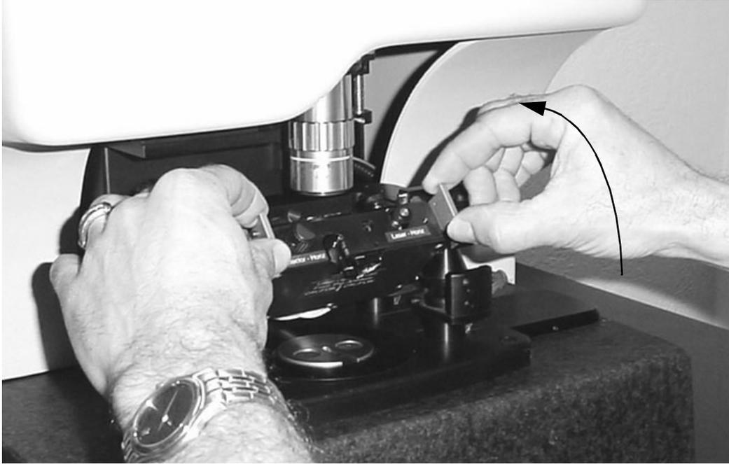
Figure 3.15. Rotate the scanner head.
