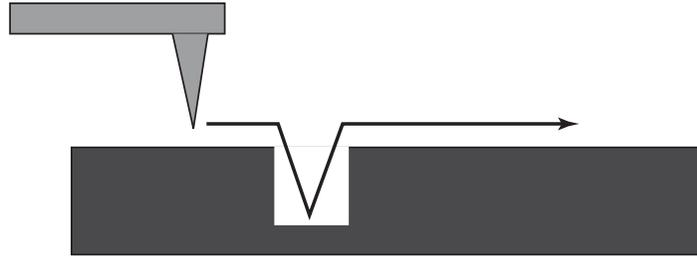
**Figure A.3.** AFM probe scanning over a depression in the surface topography.
