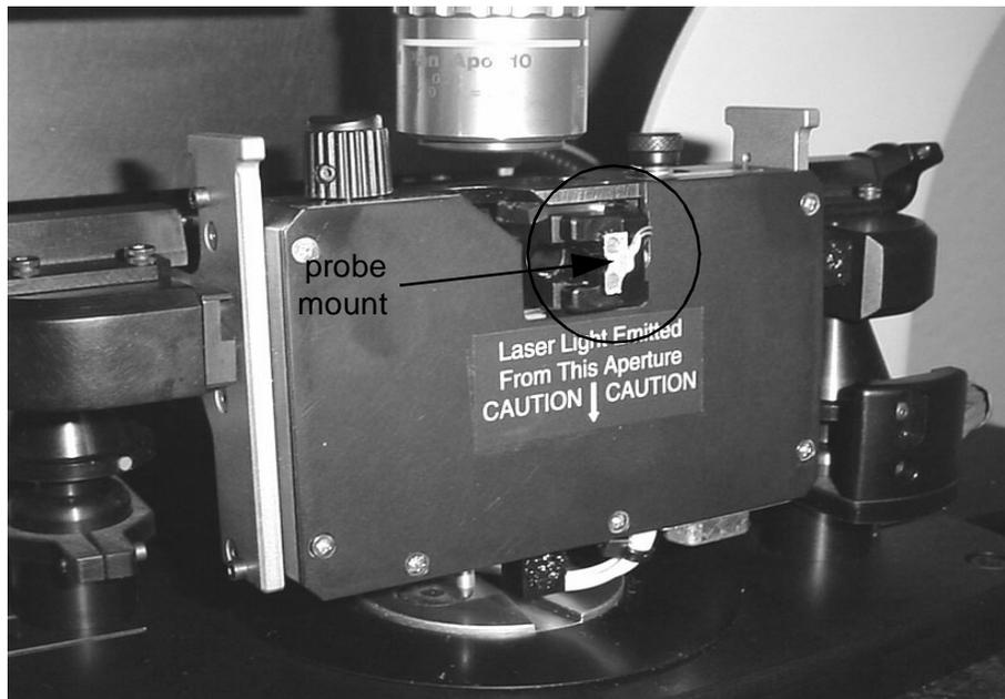
Figure 2.18. Probe exchange position.
