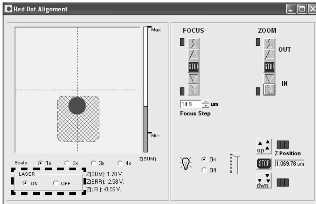
Figure 2.14. Turning off the laser.
