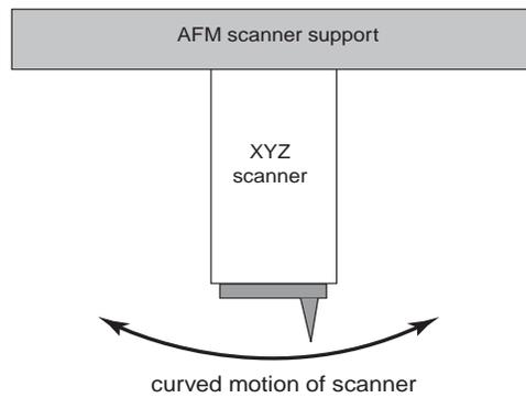
**Figure A.12.** Nonlinear Z scanner motion.
