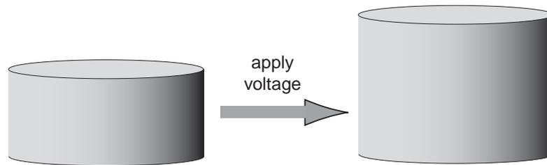
**Figure b.** When a voltage is applied to the top and bottom surface of the piezoelectric disc, the disc expands.
