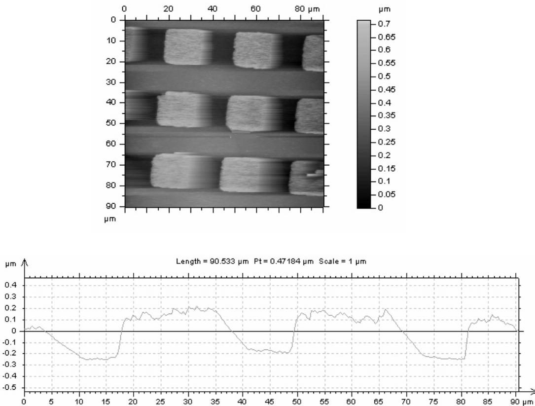
**Figure A.6.** AFM image of a semiconductor test pattern and the line profile showing an artifact. Scan size: 91 X 91  $\mu\text{m}$ .
