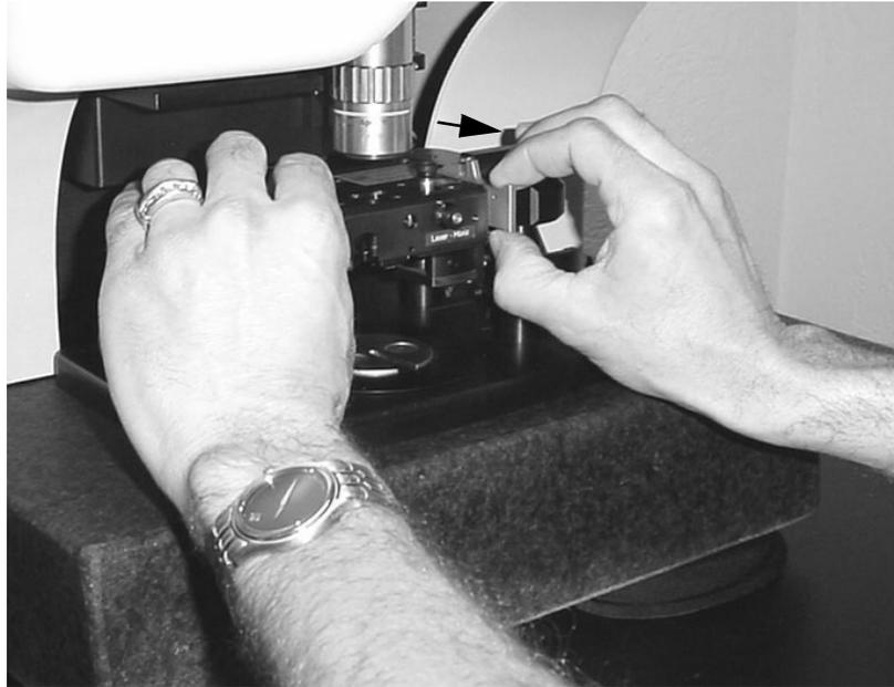
**Figure 2.16.** Slide the scanner head toward you.
