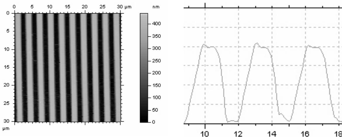
**Figure A.15.** This AFM image of a test pattern appears to have no artifacts, but the line profile shows overshoot at the top of each line.
