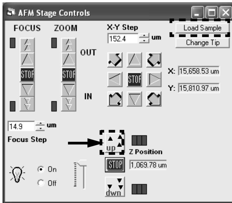
Figure 3.8. Raise the probe tip away from the sample.
