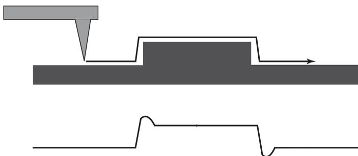
**Figure A.14.** Overshoot in scan (top) is apparent in the line profile (bottom).
