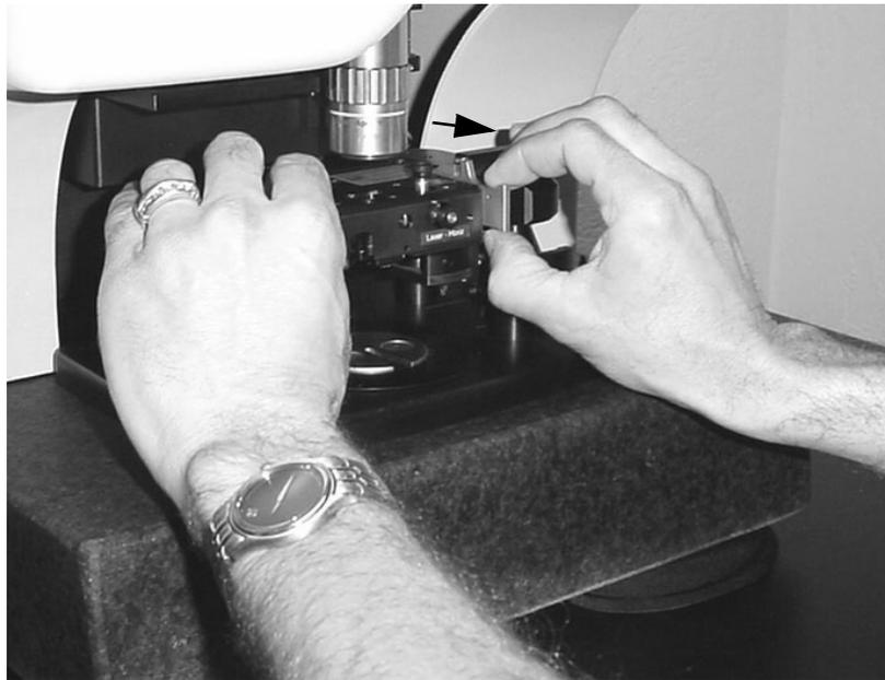
**Figure 3.14.** Slide the scanner head toward you.
