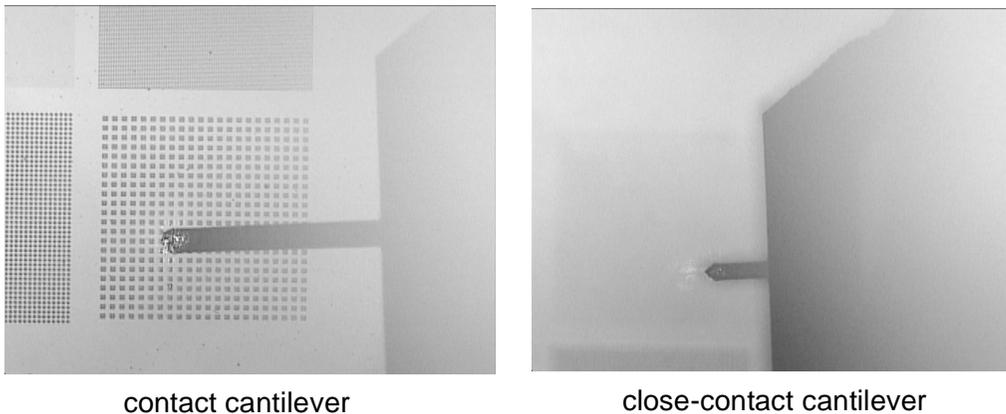
**Figure 1.7.** The two cantilever types, as seen on the video microscope monitor.
