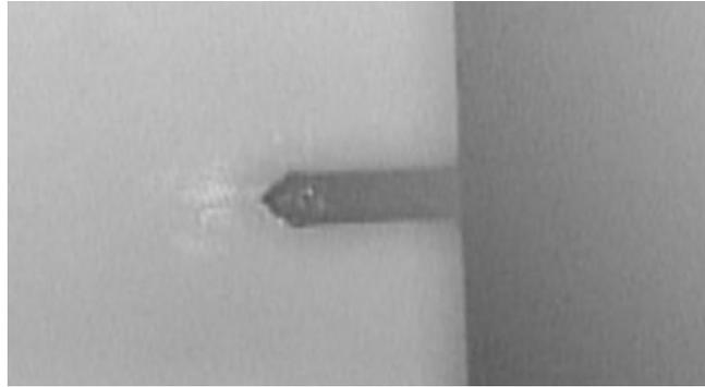
Figure 3.24. Centering the laser spot on the cantilever.
