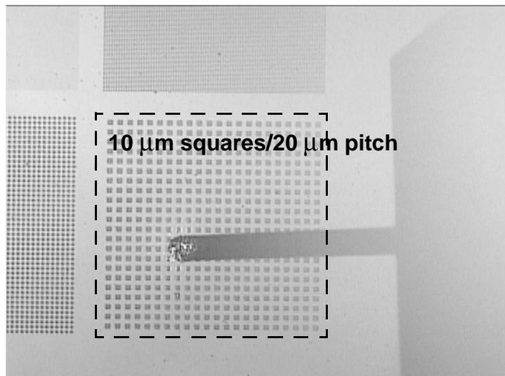
Figure 2.29. Positioning the probe over the scan area.
