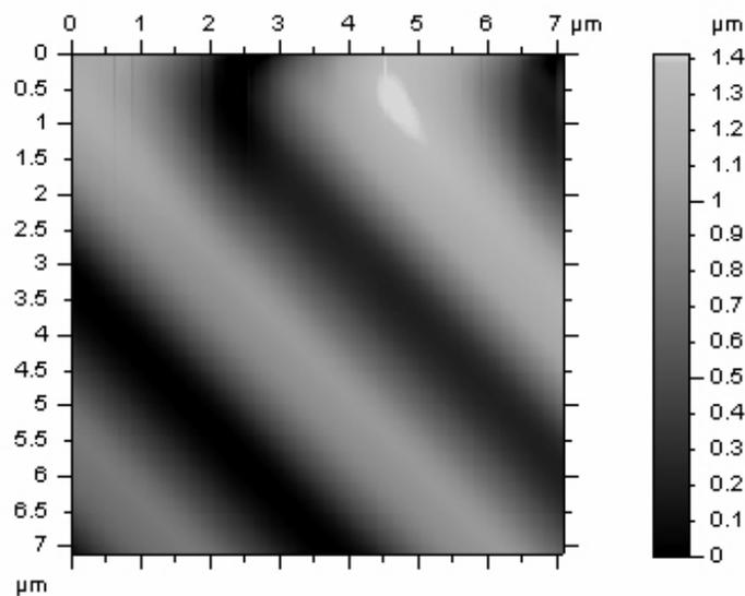
**Figure A.17.** Zoomed image showing a distortion at the beginning of the scan (scan angle:  $45^\circ$ ).
