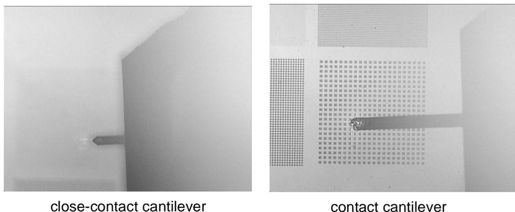
**Figure 2.25.** Contact vs. close-contact probes.
