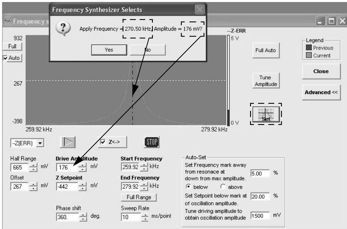
**Figure 3.29.** Confirm the frequency and drive amplitude.
