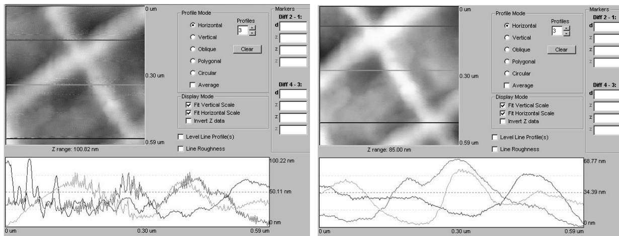
**Figure A.25.** High resolution images of a test grid with acoustic noise present in the room (left) and without noise (right).
