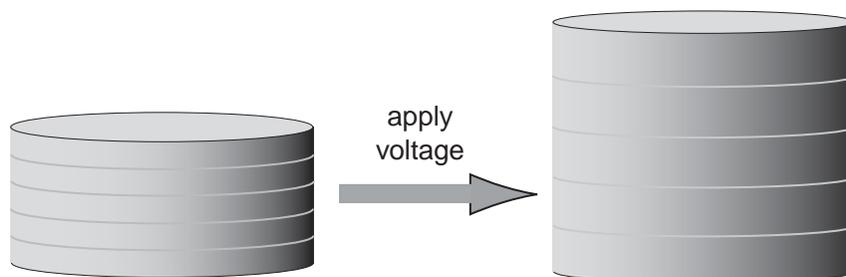
**Figure c.** When a voltage is applied to the top and bottom surface of a stack of piezoelectric disks, the entire stack expands.
