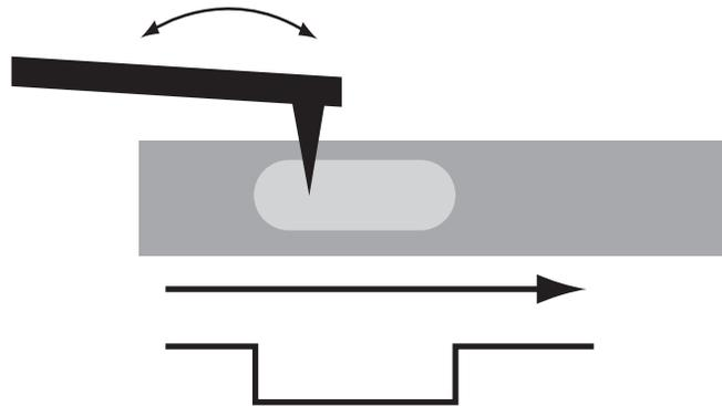
**Figure i.** Torsion mode: changes in the torsion of the cantilever are an indication of changes in the surface chemical composition.
