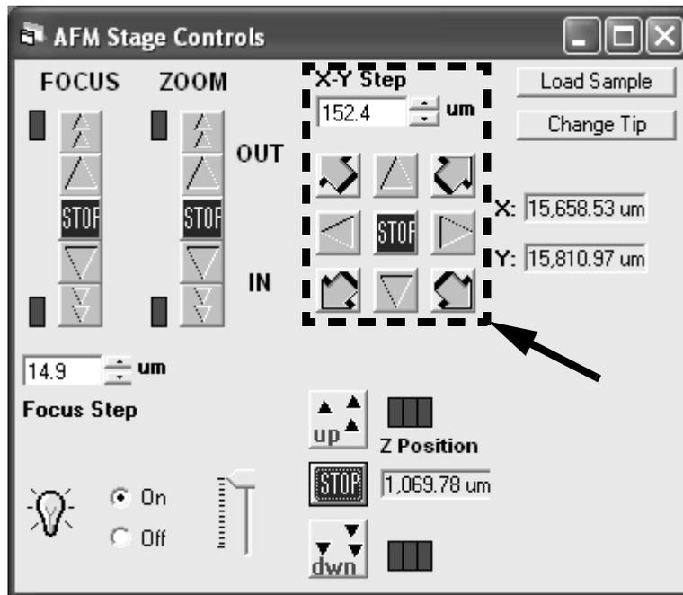
Figure 3.31. X-Y stage controls.
