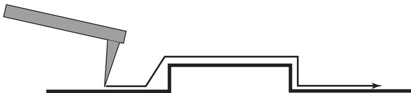
**Figure A.8.** A sharp probe scanning at an angle.
