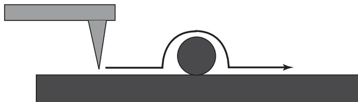
**Figure A.1.** AFM probe scanning over a spherical surface feature.
