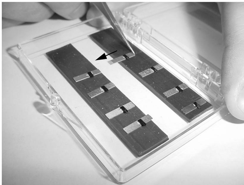
**Figure 2.20.** Nudge the probe into position.
