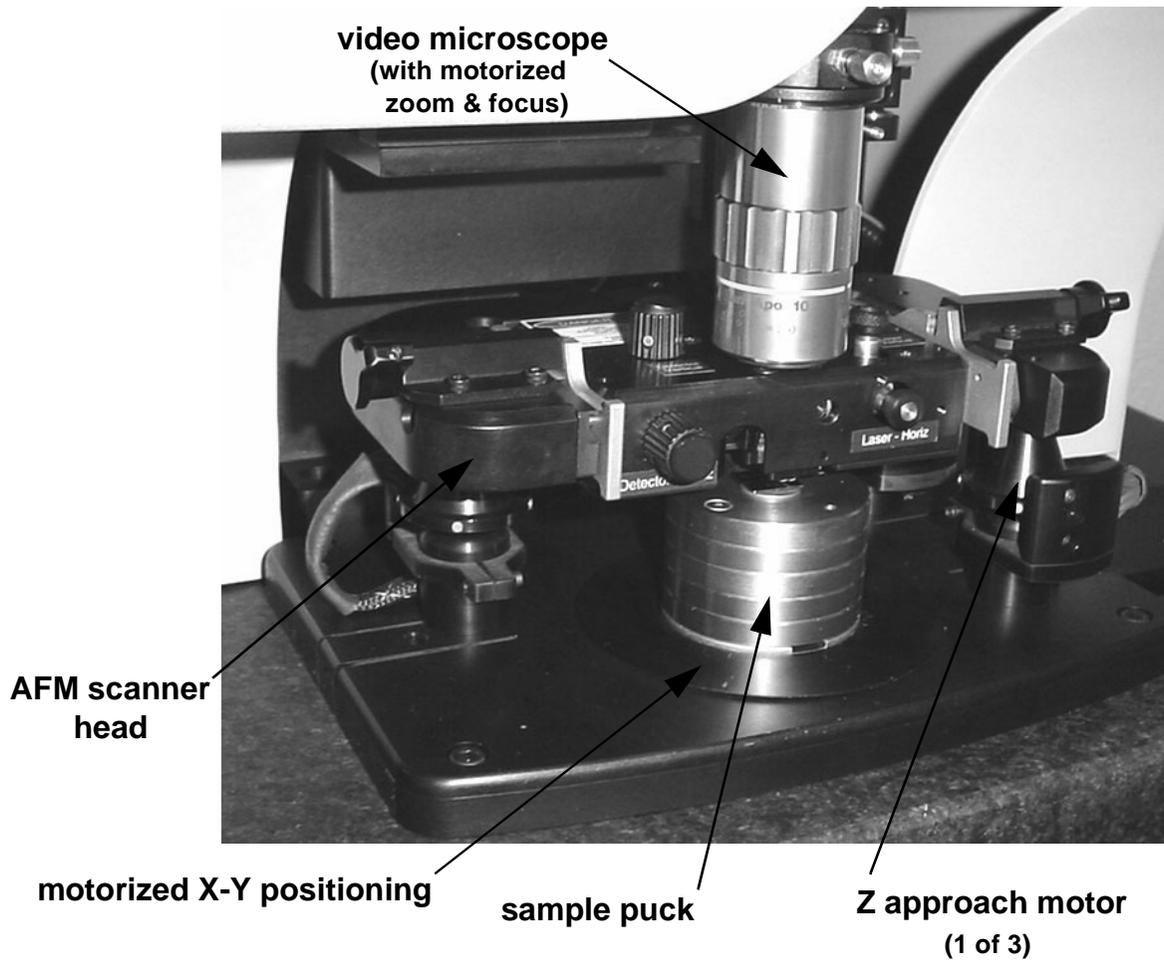
Figure 1.2. Stage components.
