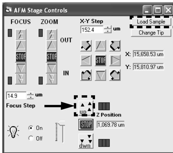
Figure 2.8. Raise the probe tip away from the sample.
